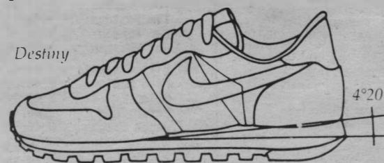
The Destiny has a midsole and wedge scaled for cushion as well as the same degree of heel lift in each size.
